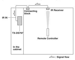
The IR IN input allows you to control the TX-DS797 from the remote zone (Zone 2) with the remote controller even though the remote zone is physically separated. The diagram below shows how to make the proper connections for the remote zone.
